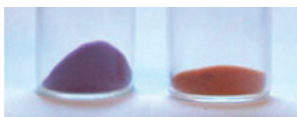
Figure 4. Photograph showing silica gel containing adsorbed 1\cdot(\text{CH}_3\text{CO}_2\text{H})_2 in contact with air in the absence (left) and the presence of 50 ppm of CO (right).
